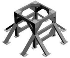
The solution: Kanya heavy-duty aluminum extrusion or t-slots as they are non-magnetic. In addition, all the connectors, isolation pads and floor mounting plates were made from 304L stainless steel. The aluminum extrusion design is rigid and this feature minimized flex in the base, which was another specification.
