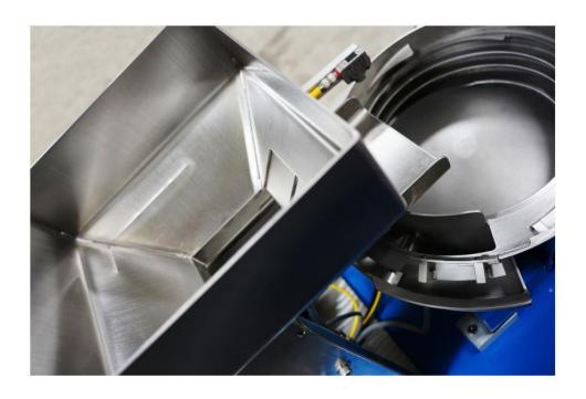
Prefeeders come in a variety of styles. Depending on the layout and product, Hoosier Feeder Co. can integrate either an elevator or hopper to handle the bulk delivery of parts to the feeder and optimize the efficiency of the entire system.
