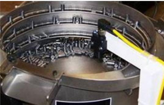
The majority of vibratory feeders will be shipped with tool steel tracks removed and stainless steel temporary springs on the inline drivers to prevent damage in transit. When you receive the feeding machine, you must install the tool steel inline tracks, remove the "shipping springs", and align the inline track and bowl discharge. If you take care during this step, the feeder bowl will function much more smoothly.
