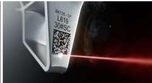
DataMatrix Laser Marking
